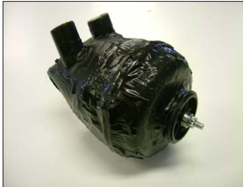
Figure 4. Modified turbocharger unit with circulation control primary plenum chamber
