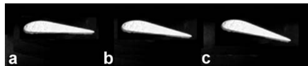
Figure 6 Low aspect ratio rotor blades for control at various attitudes (a) 0^\circ (b) 5^\circ (c) 10^\circ .
