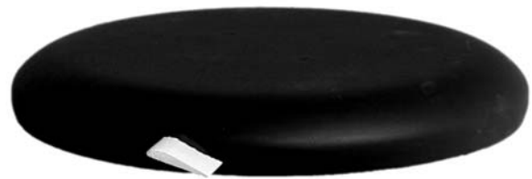
Figure 5 Low aspect ratio rotor blade, at 10^\circ attitude with respect to the disc planform.
