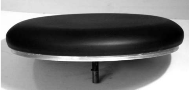
Figure 7 Variable rim height device attached inside the disc rim extending the disc thickness by 7mm or h/t = 0.2 .
