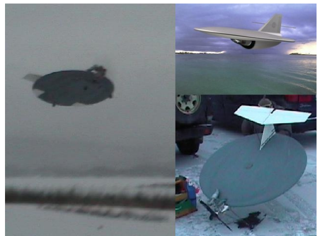
Figure 2 Photomontage of SiMiCon Rotor Craft (SRC), courtesy of SiMiCon AS. (Top Right) SRC cruise concept (Bottom Right) Circular planform aircraft flight demonstrator (Left) Demonstrator aircraft in-flight.
